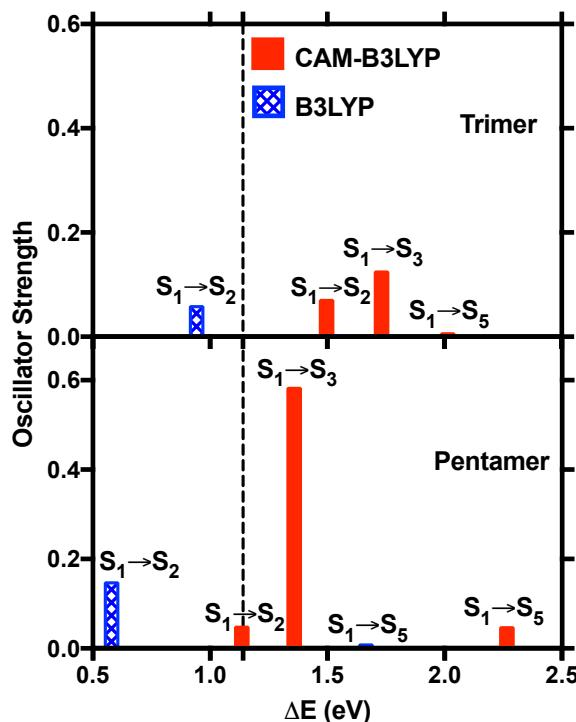
Figure S2: Calculated excitation energy of the  $S_1 \rightarrow S_n$  transitions for 3MT trimer and pentamer using B3LYP (checkered blue) and CAM-B3LYP (solid red) functionals. The vertical dashed line indicates the experimental ESA energy of P3HT.<sup>19</sup>
