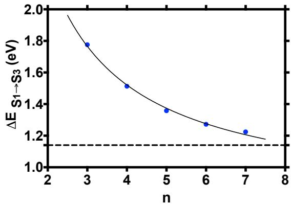
Figure S6: Calculated excitation energy of the  $S_1 \rightarrow S_3$  transition for 3MT oligomers of length  $n = 3$  to 7 obtained from the relaxed  $S_1$  molecular geometry (blue data points). The solid curve shows the  $1/n$  dependence of the excitation energy. The horizontal dashed line indicates the experimental ESA energy of P3HT.<sup>19</sup>
